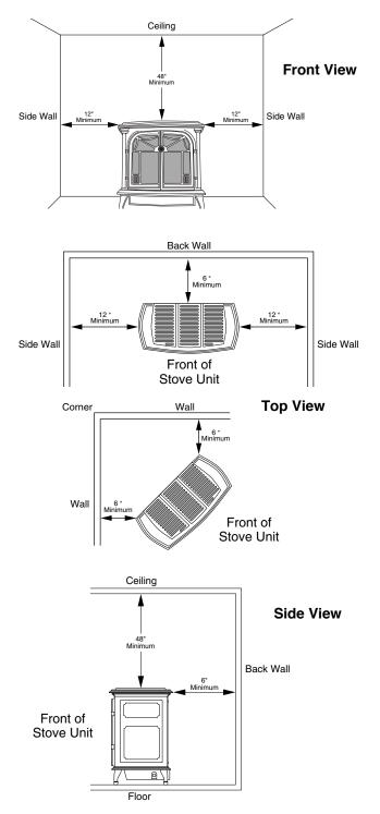
Figure 5 - Minimum Clearance to Walls and Ceiling (Stove May Vary Depending on Model)
